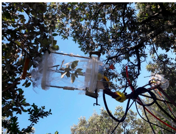
Figure 2. Photo of the branch chamber used during the Puechabon field experiment.
